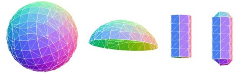
Figure 2. 3D simple objects created using marching cubes, with low quality (resolution) and sharp edges.
