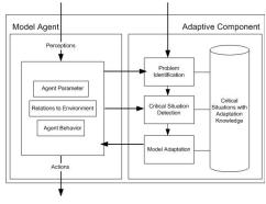
Figure 2: Architecture of a self-debugging agent with both nominal (left side) and adaptive behavior (right side).
