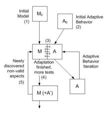
Figure 1: Adaptation-driven design process starting from an initial model  $M_0$  and a corresponding adaptive repair component  $A_0$ . After iteratively testing and adapting, an improved model is produced that may contain some built-in adaptive elements.
