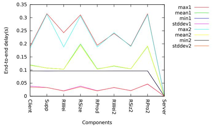
Figure 3. End-to-End delay - Scenario 1 and 2.
