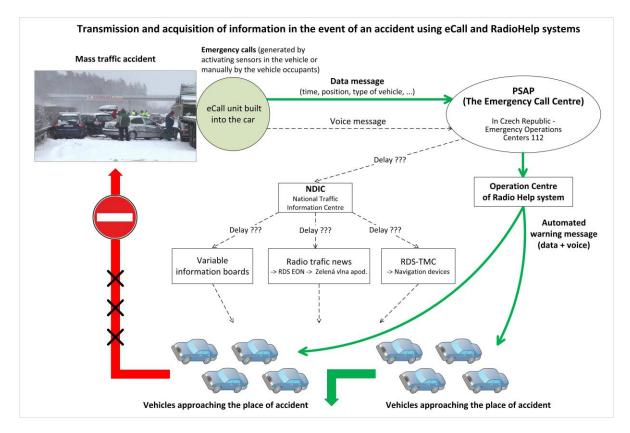
Figure 2. Transmission and acquisition of information in the event of an accident with the use of eCall and Radio-Help (Source: Authors)
