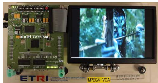
Figure 5. EVM board of multi-core SoC (MOSAIC)
