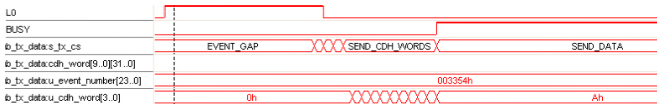
Figure 6. Timing diagram obtained using Altera signal-tap logic analyser for data transfer between RCB and DAQ.
