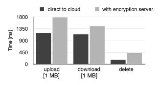
Figure 6. Diagram of average times to upload, download, and delete files with and without encryption
