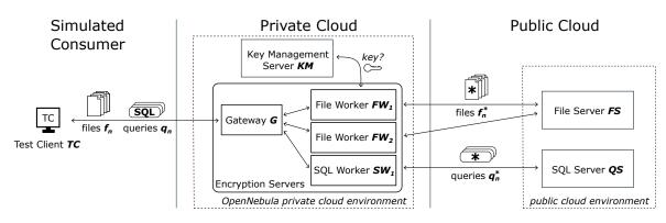
Figure 2. The implemented encryption server prototype as one core component of the proposed hybrid cloud architecture.
