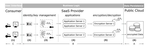
Figure 1. The hybrid cloud architecture for SaaS with an enhanced business logic layer by key management and encryption layer. Lines separate the actors and architecture layers. Dashed lines illustrate encrypted keys. Dotted lines represent a physical separation. Rounded and rectangular boxes represent virtual servers and data, respectively. A,B and C show the range of the thread scenarios.
