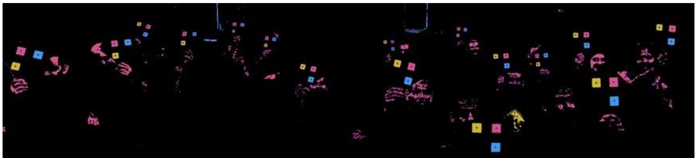
Figure 5. An example of color markers recognition. All the markers of all 16 IFS cards (see Fig. 1) were successfully recognized as color rectangles. The calculated geometrical centers of the rectangles are marked as black dots.
