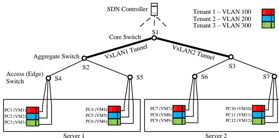
Figure 1. A multi-tenancy architecture used in both 1) VMWare/Mininet and 2) GNS3 tools.
