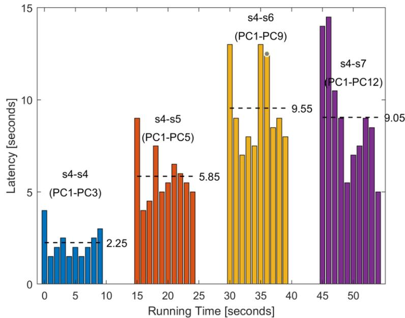
Figure 4. Latency in inter-VLAN communications
