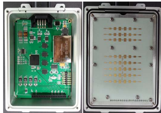
Figure 2. Signal processing module and transceiver of the Developed BSD/LCA radar system
