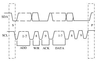
Figure 1. Data transfer on I2C bus
