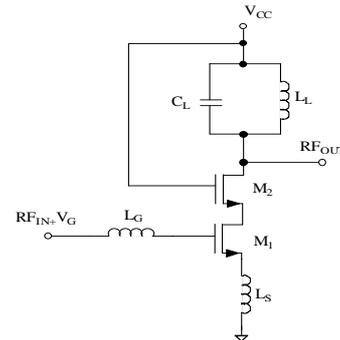
Figure 3: Circuit of the Low Noise Cascode Amplifier
