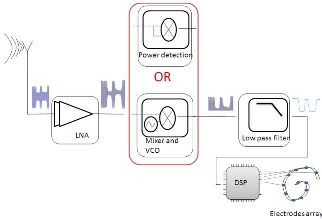
Figure 2 : Transmitter architecture overview, with signal outputs in color
