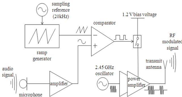
Figure 1: Transmitter architecture (redrawn from)
