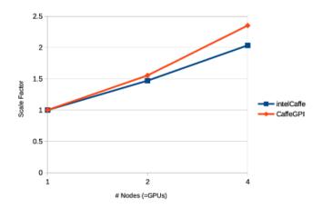
Figure 6. Scaling results for AlexNet with an overall batch size of 256 on distributed nodes with single GPUs interconnected via Infiniband. Based on Intel<sup>TM</sup>Caffe 1.14, Cuda 8, CuDNN 5.1
