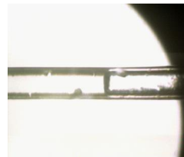
Figure 14. Video image of the meniscus in the capillary.
