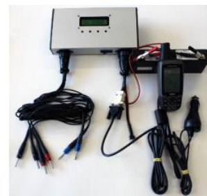
Figure 9. Electrical soil conductivity measurements system.
