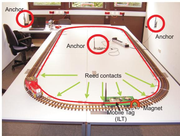
Figure 8. Indoor localization testbed for performance evaluation of the map generator
