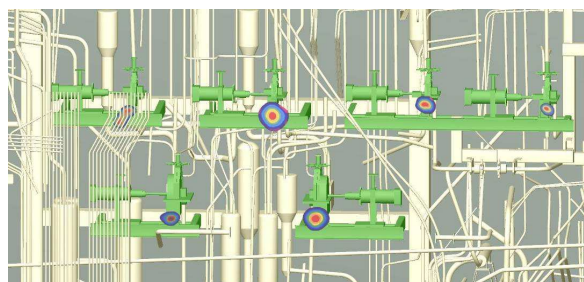
Figure 25. Hot spots on dosing wheels
