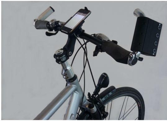
Figure 12. Chording keyboard prototype mounted on a bike handlebar. The four visible buttons correspond to the index, middle, ring and pinky fingers. The thumb button is on the other side of the prototype.
