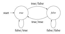
Figure 1. Automaton obtained from toggle switch program
