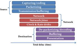
Figure 1. End-to-end causes of delay.
