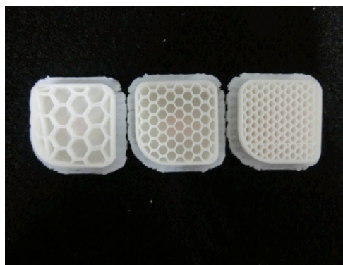
Figure 3. Photographs of inside low infill density objects.
