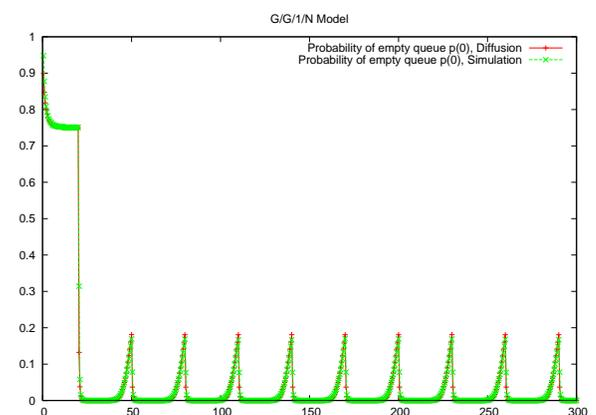
Fig. 7. Example 2: The probability  $p(0, t)$  of the empty queue, diffusion approximation and simulation results.
