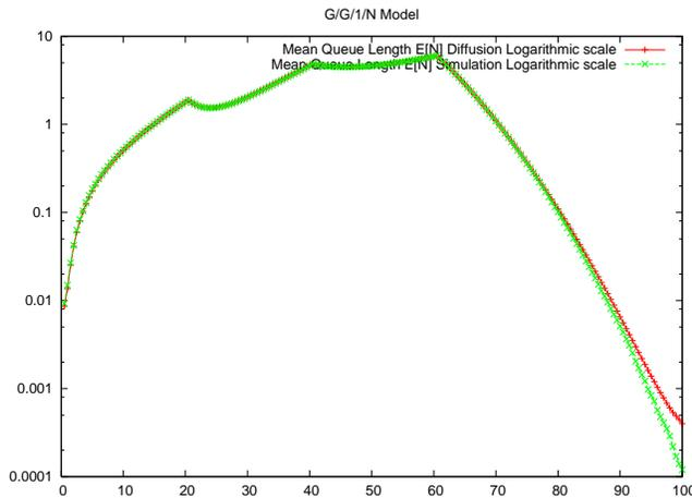
Fig. 3. Example 1: The mean number of customers (logarithmic scale) as a function of time; diffusion approximation and simulation results. .
