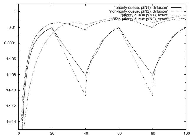
Fig. 18. Example 6: Probabilities  $p^{(1)}(N^{(1)}, t)$ ,  $p^{(2)}(N^{(2)}, t)$  that the queues of class 1 or class 2 are saturated, diffusion approximation and exact results. Logarithmic scale is chosen for better presentation of very small probabilities.
