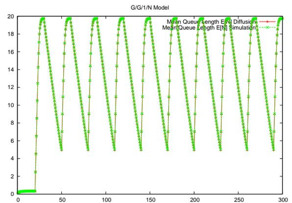
Fig. 6. Example 2: The mean number of customers as a function of time; diffusion approximation and simulation results. .
