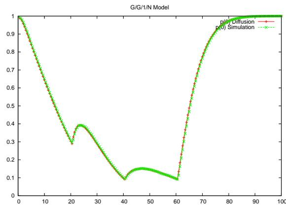
Fig. 4. Example 1: The probability  $p(0, t)$  of the empty queue, diffusion approximation and simulation results.
