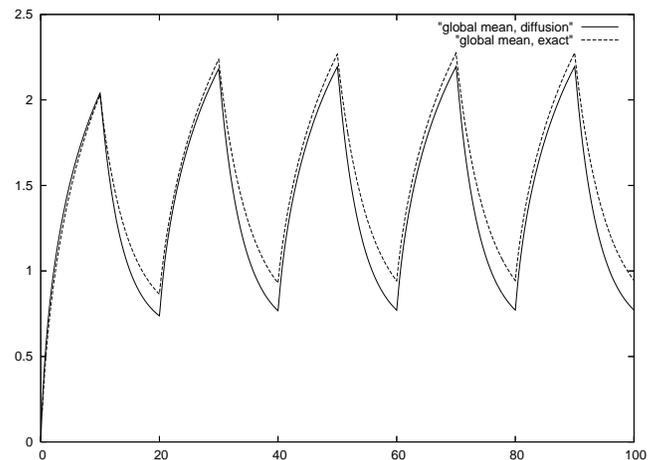
Fig. 14. Example 5: Global mean number of customers as a function of time, diffusion approximation and exact results.
