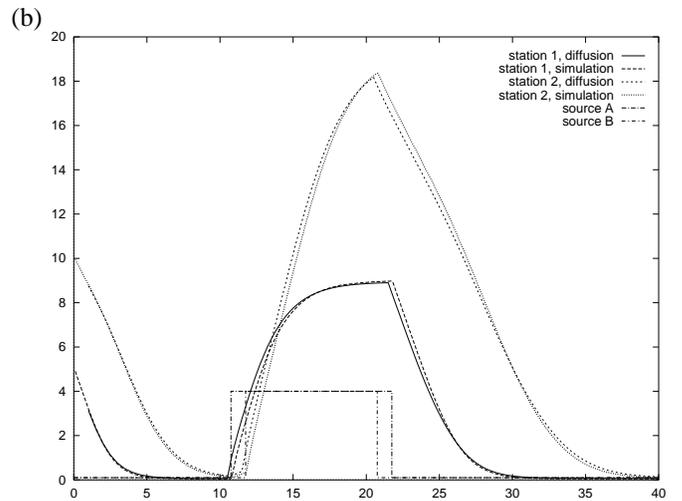
Fig. 10. (a) Example 3: The mean queue lengths of station1, station2 and station3 as a function of time — diffusion and simulation (100 000 repetitions) results; the source intensity  $\lambda(t)$  is indicated. (b) Example 4: The mean queue lengths of station1 and station2 as a function of time — diffusion and simulation (100 000 repetitions) results; the source intensities  $\lambda_A(t)$ ,  $\lambda_B(t)$  are indicated.
