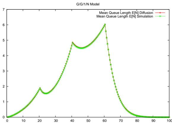
Fig. 2. Example 1: The mean number of customers as a function of time; diffusion approximation and simulation results. .
