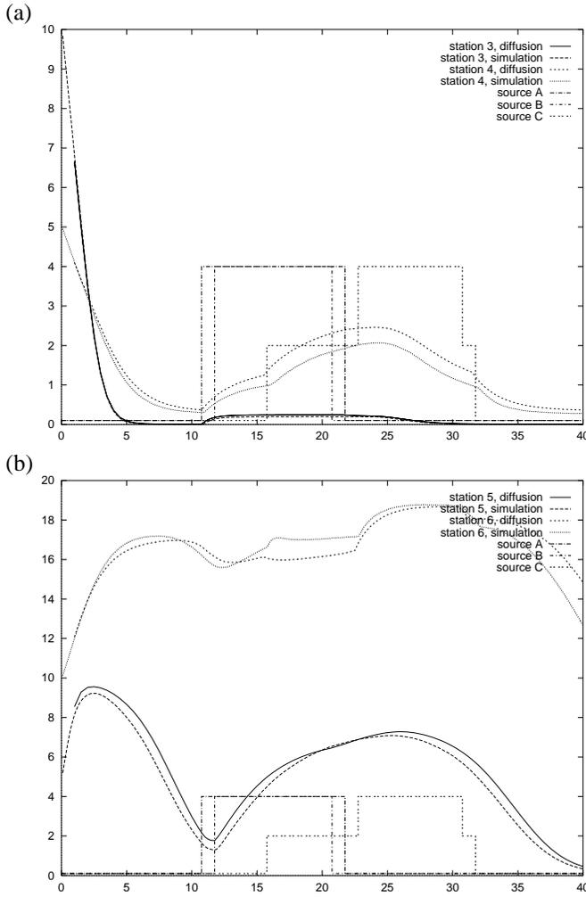
Fig. 11. Example 4: The mean queue lengths of station3 and station4 (a) and of station5 and station6 (b)
