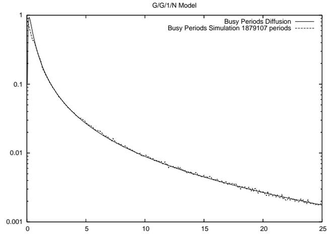
Fig. 12. M/M/1/20 queue,  $\rho = 0.75$ , busy period diffusion approximation compared with simulation (histogram of over 1.8 million samples).
