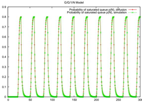
Fig. 8. Example 2: The probability  $p(N, t)$  of the saturated queue, diffusion approximation and simulation results.
