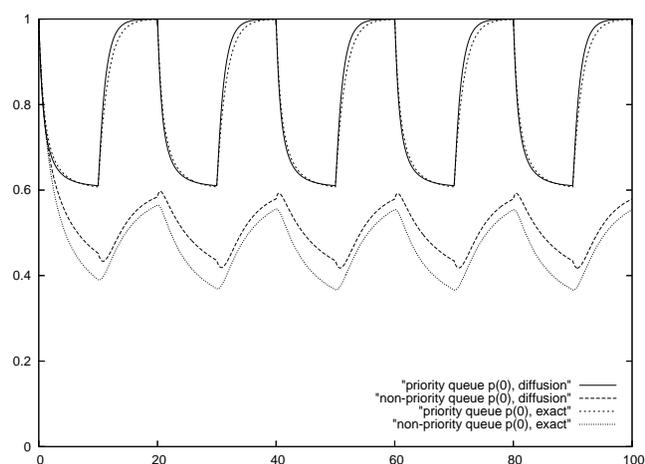
Fig. 17. Example 5: Probabilities  $p^{(1)}(0, t)$ ,  $p^{(2)}(0, t)$  that the queues of class 1 or class 2 are empty, diffusion approximation and exact results.
