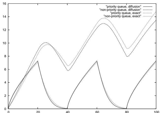
Fig. 15. Example 6: The mean number of customers as a function of time for the first and second priority levels, diffusion approximation and exact results.
