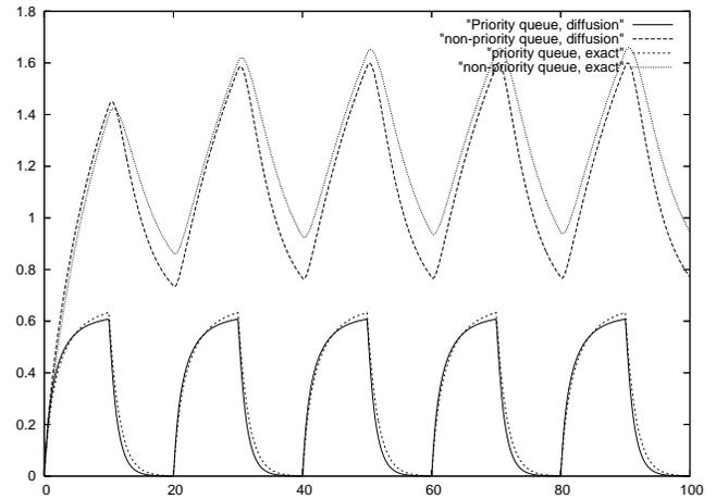
Fig. 13. Example 5: Mean number of customers as a function of time for the first and second priority levels, diffusion approximation and exact results
