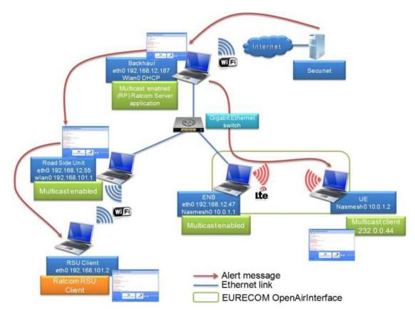
Figure 11. Experimental testbed setup for the demonstration
