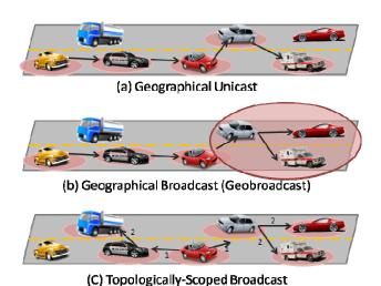
Figure 6. Types of V2V communication, (a) geographical unicast (b) Geobroadcast (c) Topologically-scoped broadcast
