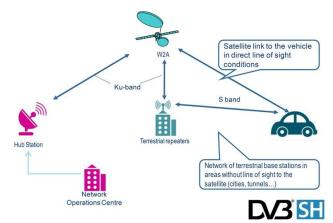
Figure 2. DVB-SH broadcast network architecture
