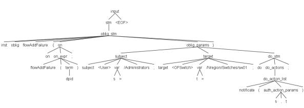
Figure 7. The AST tree for Listing 16 example
