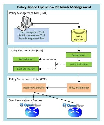
Figure 4. The Policy-Based OpenFlow Network Manager architecture
