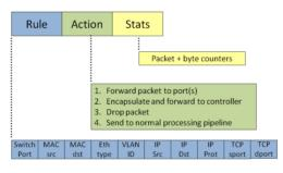
Figure 2. The OpenFlow Flow Entry [13]
