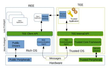
Figure 1. Standard TEE architecture
