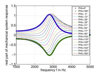
Figure 3. Influence of a varying reference phase onto real part of simulated mechanical system response, leading to falsely interpreted resonance frequency values (extremal value frequency in plot).
