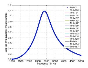
Figure 4. Advantage of combining two measurements with 90° phase difference - the calculated magnitude is independent from an unknown phase angle of excitation and measurement path.
