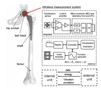
Figure 2. Overview of the diagnostic measurement system.
