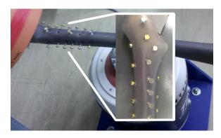
Figure 6. Measurement example with a prosthesis integrated in an artificial bone allowing an adjustable state of anchorage.
