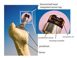
Figure 1. Medical wireless system (cross sectional cut) integrated in the femoral head of the hip implant.
