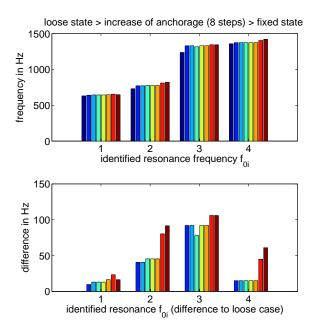
Figure 9. First four extracted resonances as identified with the diagnosis system under the influence of a step-by-step increase of prosthesis fixation (individual bars). The top plot shows the absolute frequency value for each fixation step. The bottom plot shows the absolute difference to the initial loose state.
