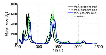
Figure 8. Calculated magnitude of several measurements on the same mechanic system with varied prosthesis anchorage state.
