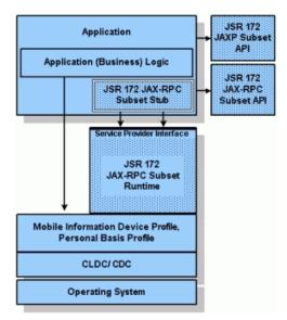
Figure 2. A typical JSR 172 based application architecture
