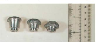
Figure 7. Deformed 6061-T6 aluminum projectiles after perforation 0.125, 0.25, and 0.5 inch thick (leftto- right) aluminum targets.
