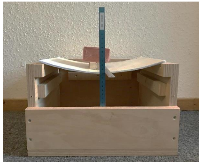
Figure 3. Sag test basic test setup with test weight.
