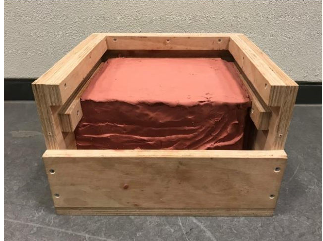
Figure 4. Shooting-box filled with plasticine. Inner dimensions: 250 mm x 300 mm x 15 mm.
