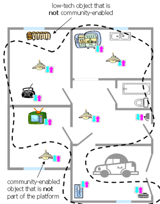
Figure 1. An indicative object community: bidirectional arrows indicate community-enabled objects, the dashed line around objects indicates the boundary of the community.
