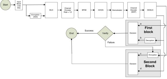
Figure 2. Error correction system using block cypher.
