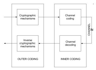
Figure 1. Cryptography and channel coding as concatenated codes.
