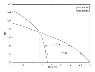
Figure 4. BER versus  $E_b/N_0$  for error correction system with and without cryptography.
