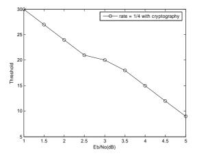
Figure 3. Threshold versus  $E_b/N_0$  for error correction system using cryptography.
