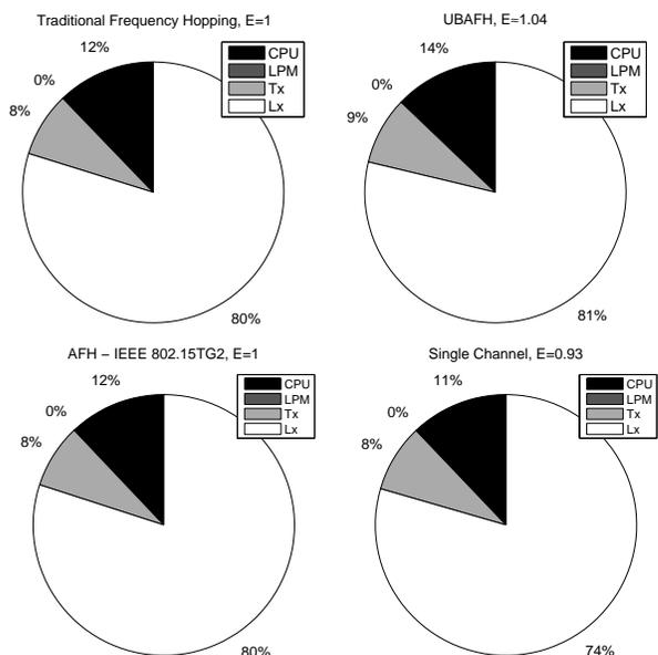
Fig. 3. Relative energy consumption in the four different energy states of the two node system for FH, UBAFH, AFH and Single Channel scheme in interference free conditions. Note that percentages of UBAFH and of the Single Channel scheme sum up to 104% and 93% respectively since we normalized the obtained values to the energy consumption of FH.
