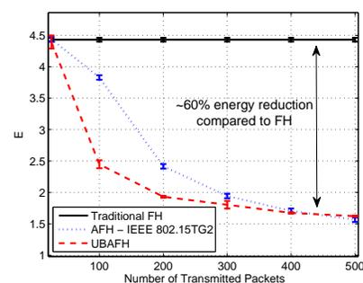
Fig. 7. Results for Scenario 3. Average energy per packet for  $p = 0.4$  (top) and  $p = 0.8$  (bottom).
