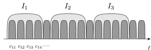
Fig. 4. Interference Scenario. Each interfering carrier  $I_i$  induces a certain packet error probability over the overlapping IEEE 802.15.4 channels.
