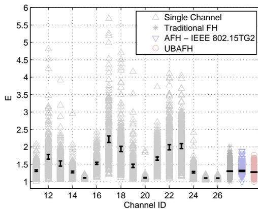
Fig. 10. Average Energy per packet for the single channel approach and for the three considered frequency hopping schemes. Results are obtained transmitting  $N = 100$  packets. 95% confidence intervals are also shown.
