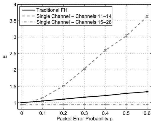
Fig. 8. Average Energy per packet as a function of the experienced packet error probability for frequency hopping and single channel scheme. Results are obtained considering  $N = 100$  packets.
