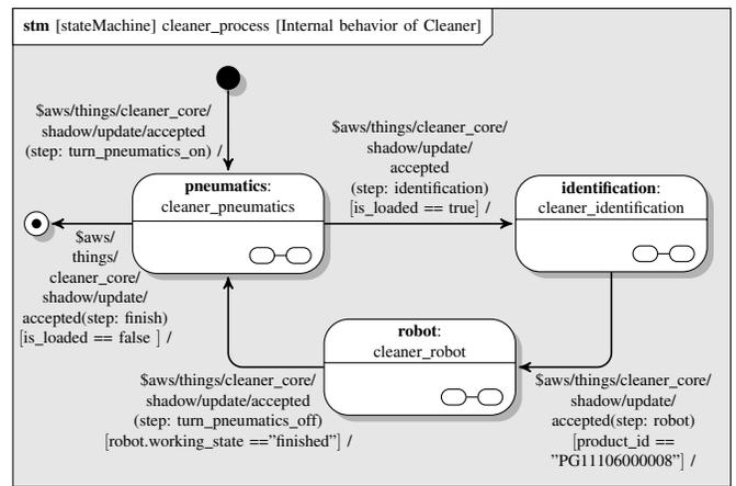
Figure 4. State machine of the *Cleaning* subprocess.
