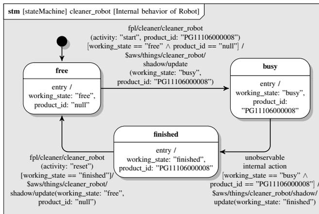
Figure 7. Sub-state machine cleaner\_robot of the *Cleaning* subprocess.
