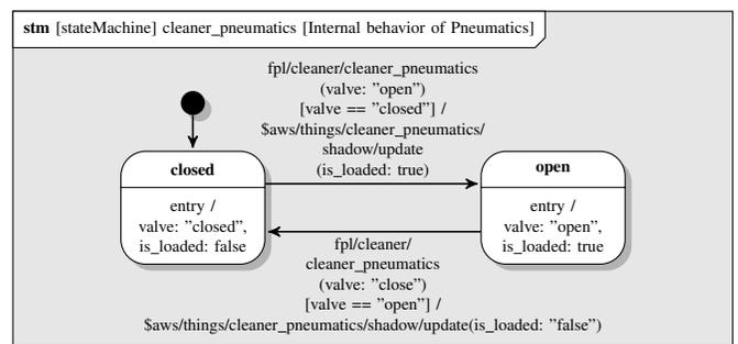
Figure 5. Sub-state machine *cleaner\_pneumatics* of the *Cleaning* subprocess.
