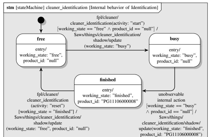
Figure 6. Sub-state machine *cleaner\_identification* of the *Cleaning* subprocess.
