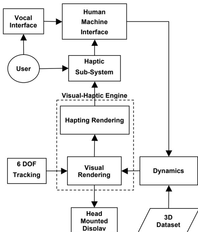
Figure 2. Schematic view of the system's architecture.
