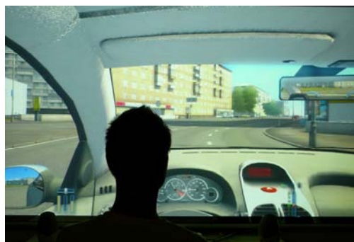
Figure 1. The car simulator consisting of a large projection screen, a steering wheel, foot pedals and a gear stick.
