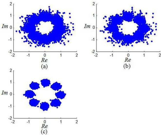
Fig. 4. Constellation diagrams of first 20000 elements of equalizer output at 8-PSK modulation. (a) VSS-MCMA, (b) CMA, (c) BML-MCMA
