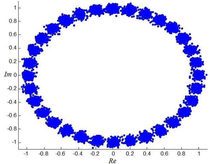
Fig. 7. Constellation diagram of first 20000 elements of BML-MCMA equalizer output at 32-PSK modulation.
