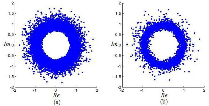
Fig. 6. Constellation diagrams of first 20000 elements of equalizer output at 32-PSK modulation. (a) VSS-MCMA, (b) CMA
