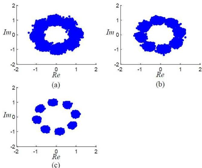
Fig. 9. Constellations of first 20000 elements of equalizer output under different buffer size values. (a)  $S = 10000$ , (b)  $S = 25000$ , (c)  $S = 50000$  symbols
