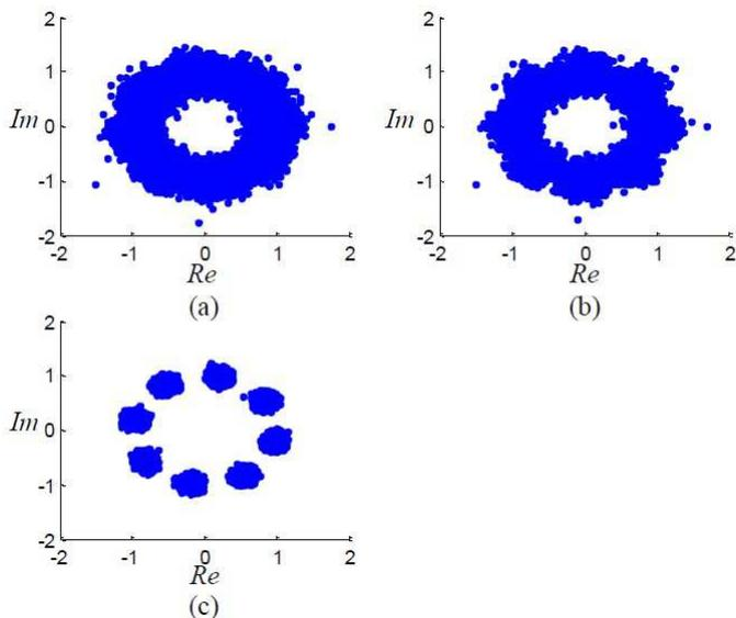
Fig. 8. Constellations of first 20000 elements of equalizer outputs at 8-PSK modulation. (a) VSS-MCMA, (b) CMA, (c) BML-MCMA
