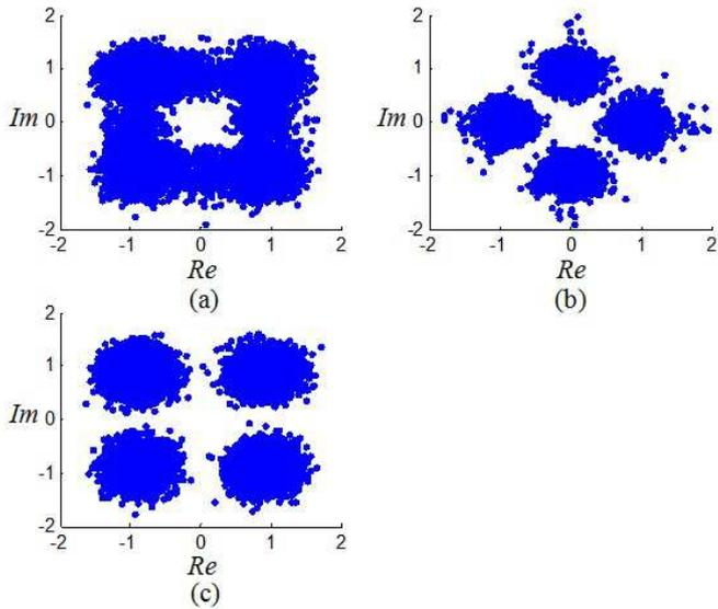
Fig. 3. Constellation diagrams of first 20000 elements of equalizer output at QPSK modulation. (a) VSS-MCMA, (b) CMA, (c) BML-MCMA
