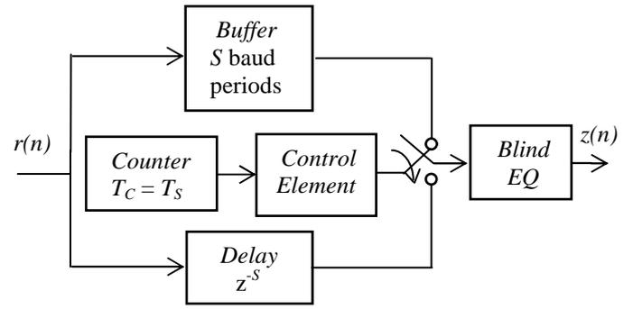
Fig. 1. Block diagram of the proposed BML – MCMA system
