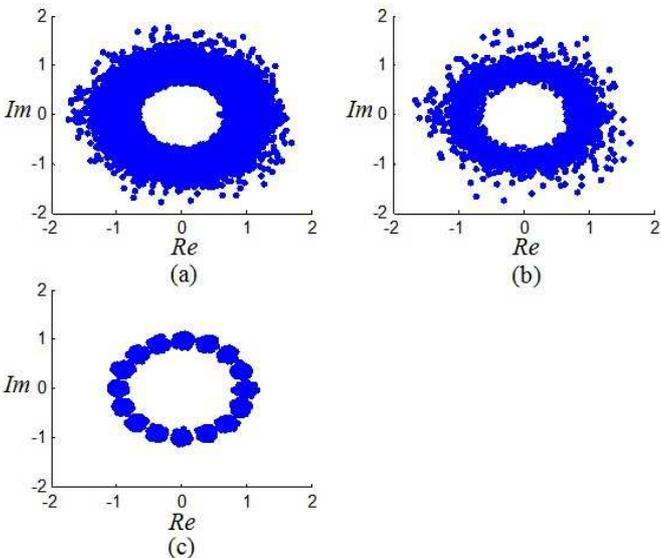
Fig. 5. Constellation diagrams of first 20000 elements of equalizer output at 16-PSK modulation. (a) VSS-MCMA, (b) CMA, (c) BML-MCMA
