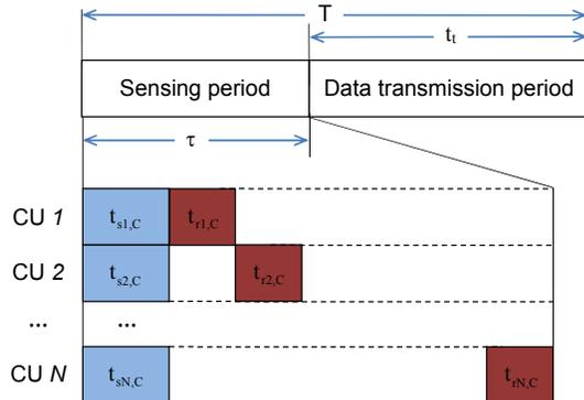
Figure 1. The time frame of conventional cooperative spectrum sensing
