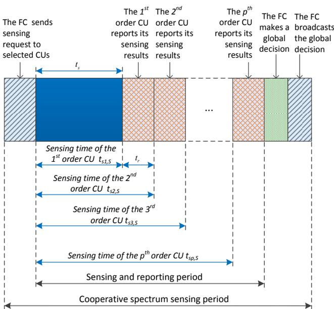
Figure 3. The time frame of the proposed scheme
