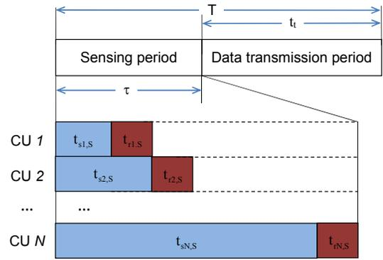
Figure 2. The time frame of superposition cooperative spectrum sensing
