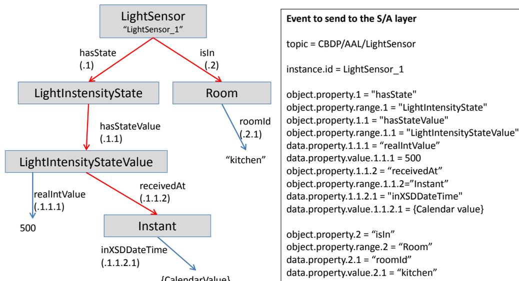
Figure 4. Example of an event containing sensor data.
