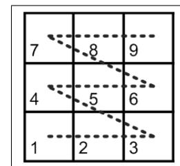
Fig. 2. X-axis linear curve in a 3x3 2-dimensional grid
