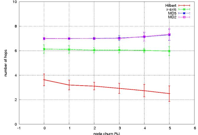
Fig. 4. Average Hop rate per cycle vs churn rate
