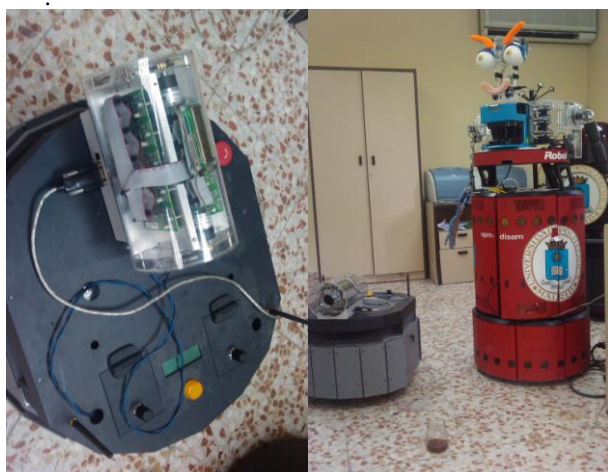
Figure 4. Urbano and the electronic nose with mobile plataform.
