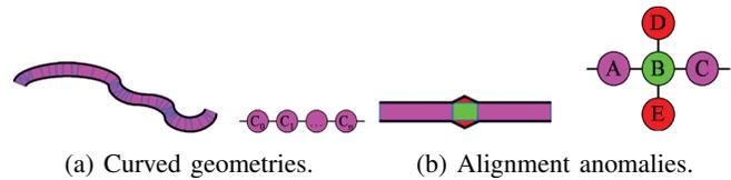
Figure 1: Cells resulting from curved geometries (a) and alignment anomalies (b) [12].
