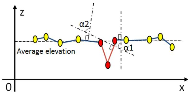
(a) Identifying elevation anomalies. Two isolated groups (in red) and angles ( $\alpha_1$  and  $\alpha_2$ ) resulting from the difference between the area-weighted normal vectors
