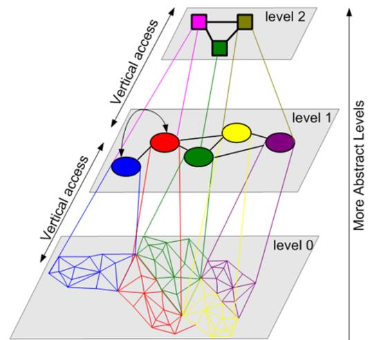
Figure 4: The topological graph extraction from space decomposition and extension into different levels using the topological abstraction.
