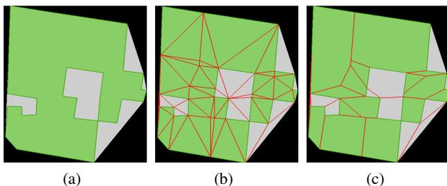
Figure 5: Illustration of the topological abstraction process with a strict convex property ( $C(gr) = 1$ ); (a) the GIS data of a complex building; (b) the exact space decomposition using CDT techniques (63 triangular cells) ; (c) the topological abstraction (28 convex polygons)
