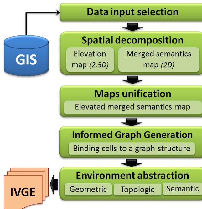
Figure 2: The IVGE global architecture of IVGE generation including the environment abstraction process.
