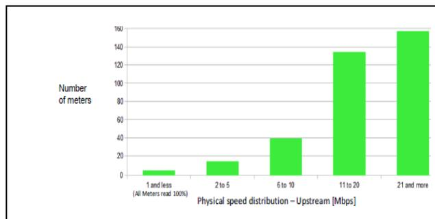
Figure 2. Physical speed distribution on a secondary substation sample equipped with BPL at CEZ as in October 2011 [17]
