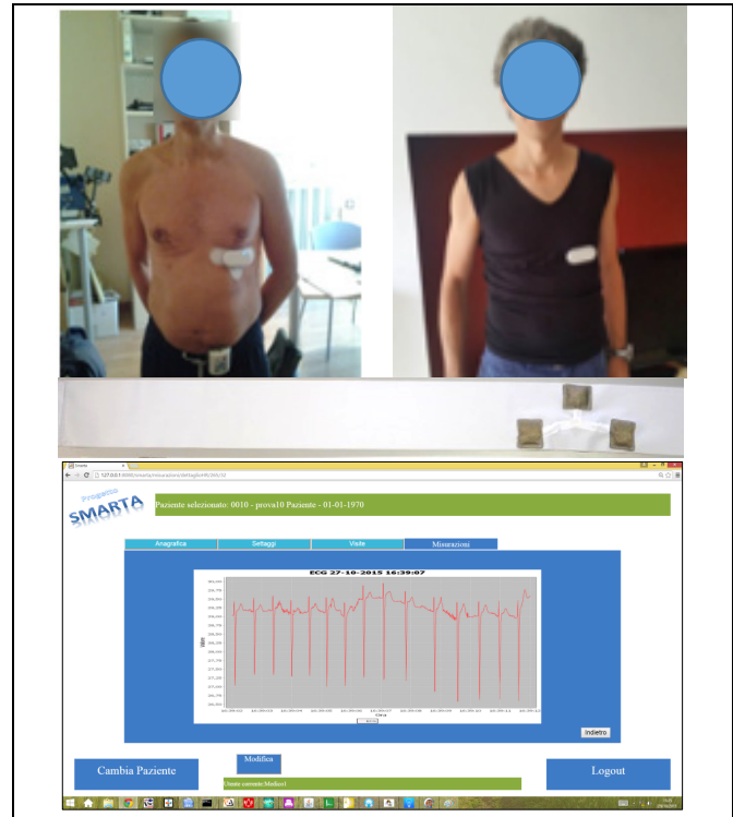
Figure 5. Wearable components of the SMARTA system (the patch, the t-shirt, the belt) and an example of acquired signal.
