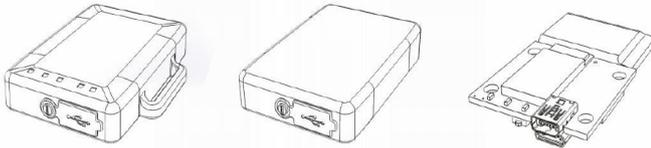
Fig. 4: Drawing of the APERTUS sensor used for axial movements.
