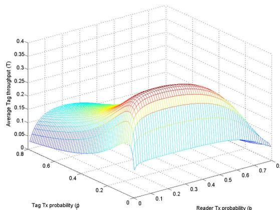
Fig. 3. Throughput ( $T$ ) vs. reader and tag transmissions probabilities ( $p_r$  and  $p_t$ ) of a symmetrical ALOHA protocol for reader and tag anti-collision assuming no interference between readers and tags.
