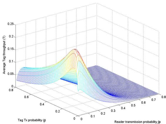
Fig. 5. Throughput ( $T$ ) vs. reader and tag transmissions probabilities ( $p_r$  and  $p_t$ ) of a symmetrical ALOHA protocol for reader and tag anti-collision assuming full interference between readers and tags.
