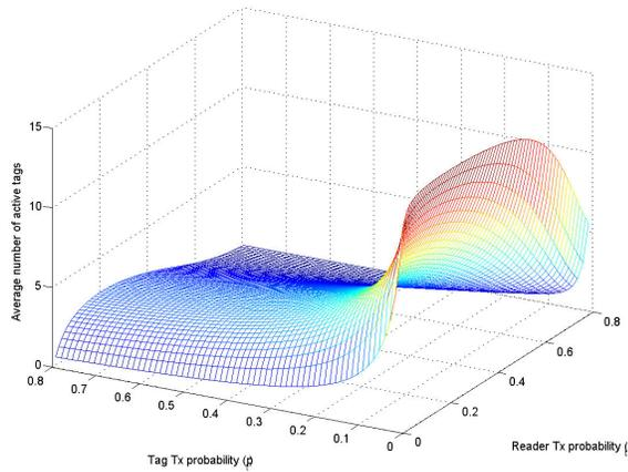
Fig. 4. Average number of active tags ( $E[|\mathcal{T}_P|]$ ) vs. reader and tag transmissions probabilities ( $p_r$  and  $p_t$ ) of a symmetrical ALOHA protocol assuming no interference between readers and tags.
