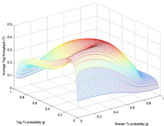
Fig. 6. Throughput ( $T$ ) vs. reader and tag transmissions probabilities ( $p_r$  and  $p_t$ ) of an asymmetrical ALOHA protocol for reader and tag anti-collision assuming no interference between readers and tags.
