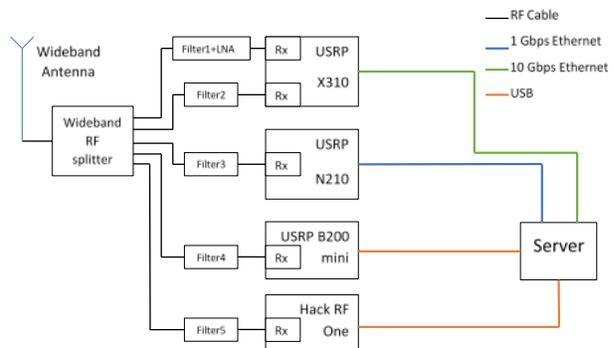
Figure 2. Preliminary architecture of the proposed spectrum occupancy evaluation system.
