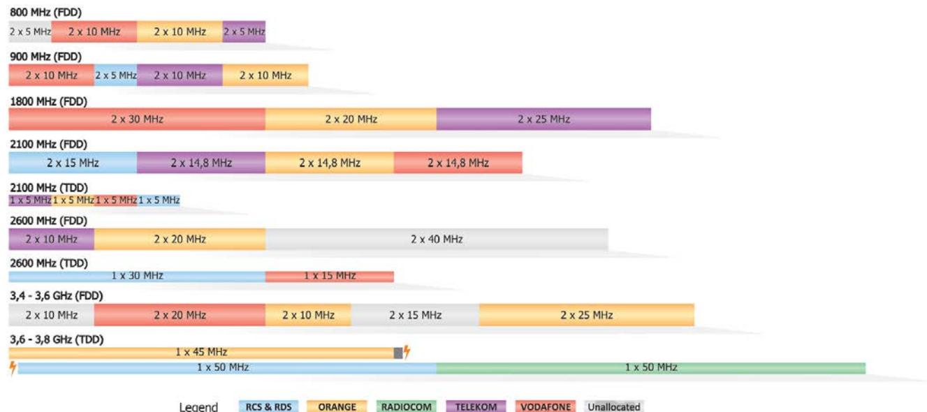
Figure 1. Allocation of spectrum resources for 2G, 3G and 4G in Romania [15]
