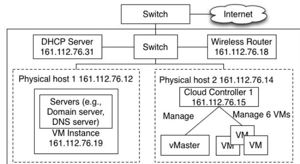
Figure 5. Network topology of cloud computing environment.
