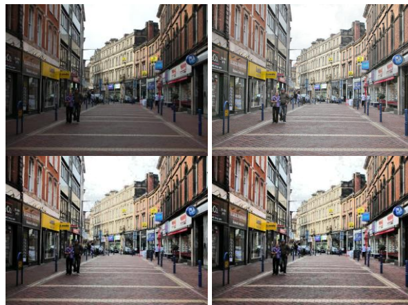
Figure 7. Resultant images from different contrast enhancement methods. From left to right, top to bottom: original image, result from our algorithm, result from HE and result from CLAHE [13].
