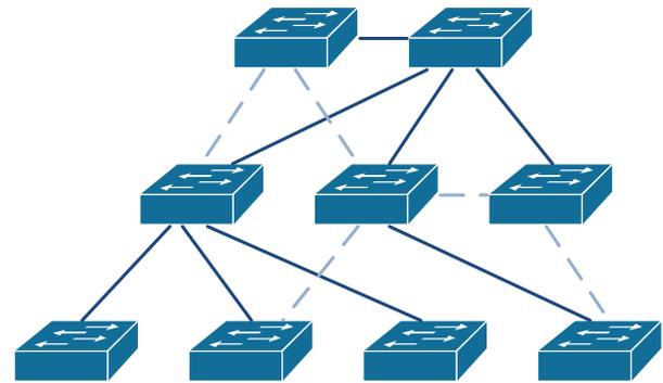
Fig. 5. RSTP redundancy is provided by stand-by links
