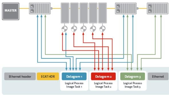
Fig. 4. Structure of the EtherCAT frame [8]
