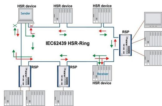
Fig. 7. HSR redundancy [14]
