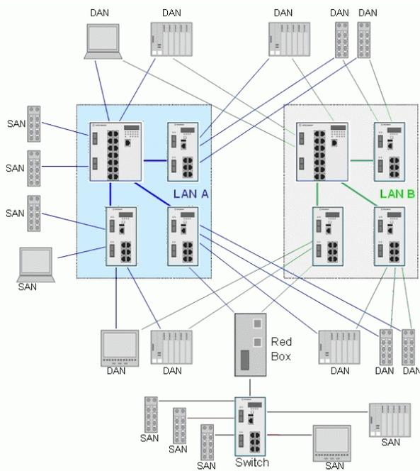
Fig. 6. PRP redundancy [14]
