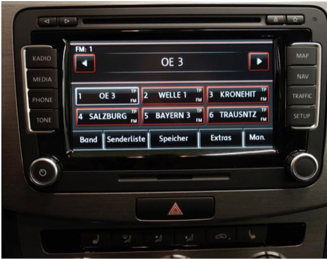
Figure 9. VW Passat dashboard which combines few physical buttons with a well-readable touch display.
