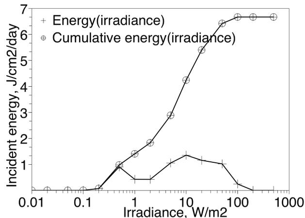
Figure 5. Harvestable energy and cumulative harvestable energy.
